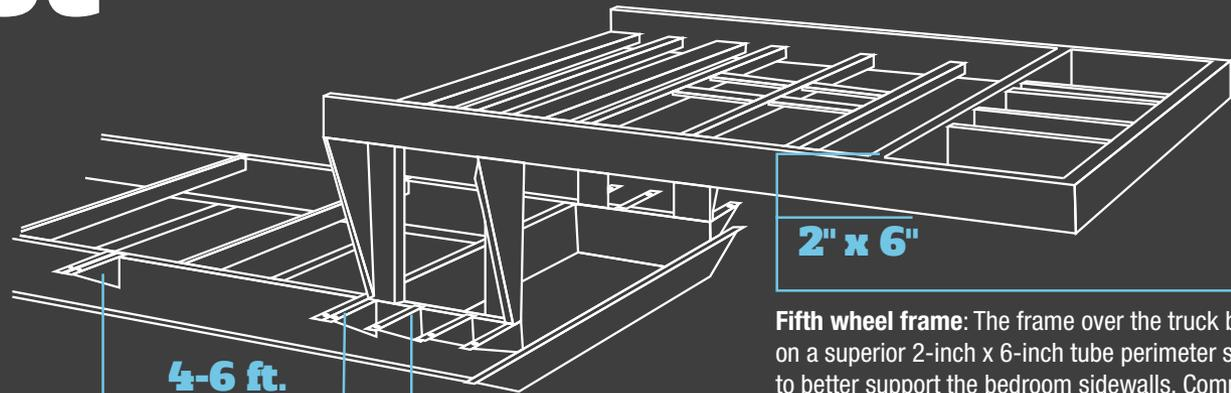
**Full-width outriggers:** We build on full-width outriggers that are spaced 4-6 feet apart (vs. 8 feet) to better support the weight of the wall.
